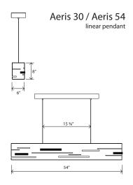
Aeris 30 dimensions - 30" x 6" x 8" H Aeris 54 dimensions - 54" x 6" x 8" H [shown] Walnut, aluminum Aeris 54 weight - 15 lbs, Aeris 30 weight - 11 lbs 72" cable standard (can be shortened in field) Energy efficient LED light source Light output - 1075 lumens [down light - 645, Up light - 430] Light color - 2700° K (warm) Color accuracy - 85+ CRI LED power consumption - 16 Watts  $Dimmable \ (use \ ELV \ or \ TRIAC \ dimmer)$ Ceiling canopy included Wood grain will vary
